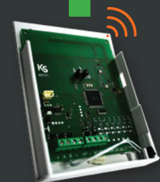
DUO 01751 Ontvangstmodule of repeater in behuizing
